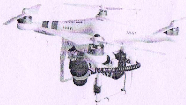
Fig. 7 Phantom 2 quadcopter with ICI thermal camera [6]
